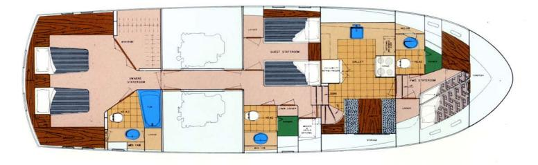
The Hatteras 58 Motor Yacht is a fiberglass, modified-vee hull yacht designed by naval architect Jack Hargrave. Power is twin 650 SHP G.M. 8V-92TI diesels, and fuel capacity is 1,030 gallons.
